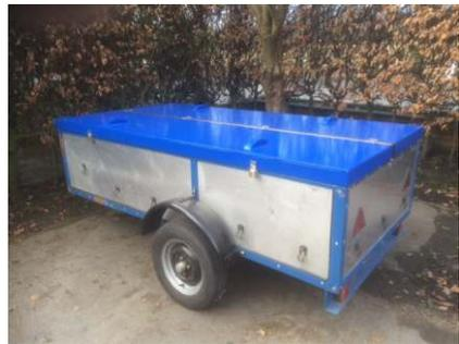
The Club trailer nears completion, it's got new suspension, lockable lids and I have removed the drop down rear door. That's been replaced with a sheet of aluminium which has been sealed with silicone. The spare wheel now resides inside the trailer. I hope we will all look smart this summer.
