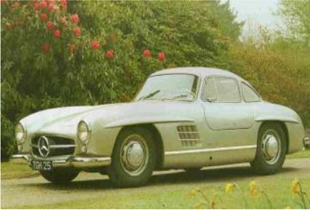
The straight six engine, canted over at fifty degrees to lower the bonnet line, was originally derived from the 300-Series 3-litre saloon. Early racers breathed through carburetors but the road going versions sported fuel-injection. The gull-wing style doors provided structural integrity to the body.
