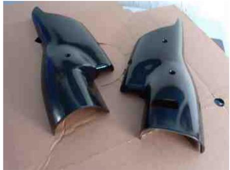
Leave the piece to dry overnight and you should have a nice, smooth, original looking item ready to be refitted. As you can see from the photos, I removed the parts (steering column cowls) from the car to work on them but, I would think you could use this method on larger parts in situ such as the dashboard.
