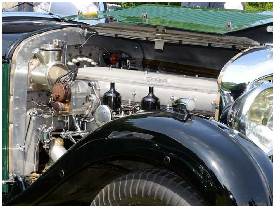
The mighty 8 litre in situ. Note the Autovac, magneto and coil ignition and spare plugs, and the diameter of that steering column!
