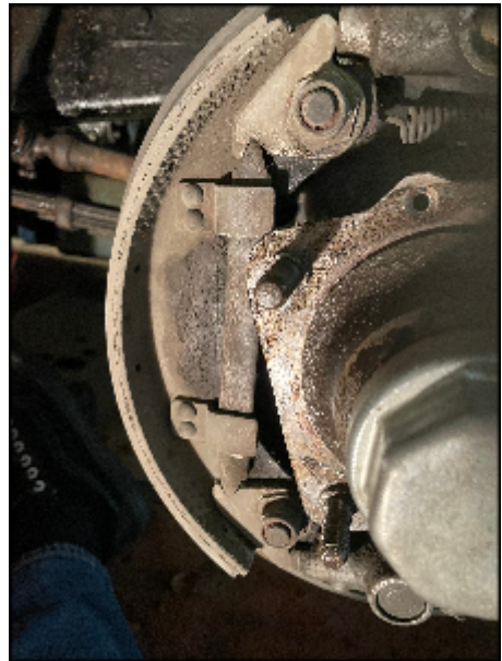
Brake work in progress on Nigel's Austin 16. Left, (Fig.1) stubborn drum finally off, and right (Fig.2) riveted self-centring device on trailing shoe.
