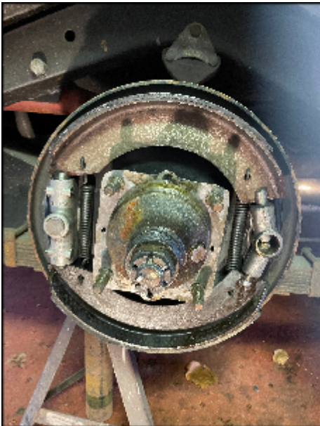
Brake work in progress on Nigel's Austin 16. Left, (Fig.1) stubborn drum finally off, and right (Fig.2) riveted self-centring device on trailing shoe.
